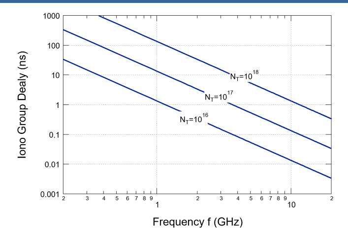
• The nominal delay for a GALILEO satellite @ 24,000 km altitude is 80 ms – this delay (smaller than 1  $\mu$ s) may appear negligible but...
