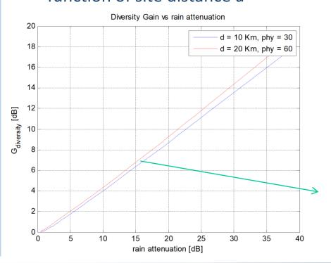
Gateway with an elevation angle of 30 degrees suffers 15 dB of attenuation for a given availability.
